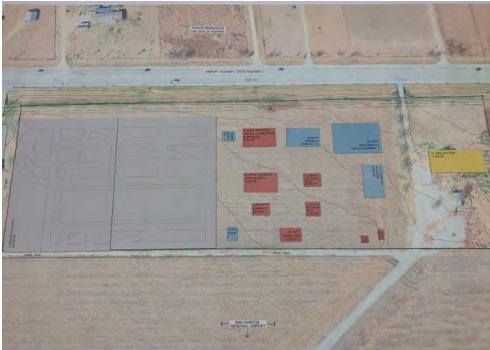
Preliminary masterplan site layout from design charette The overall fire training facility includes office/classroom building, driving skills pad, burn buildings, outdoor classrooms, and new fire station
